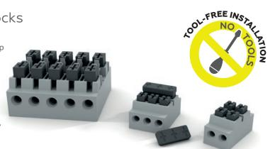
Spring-clamp technology doesn't require tools, thus making installation even simpler and quicker, and avoiding possible errors caused, with screw-type clamping units, by the application of an incorrect torque.
