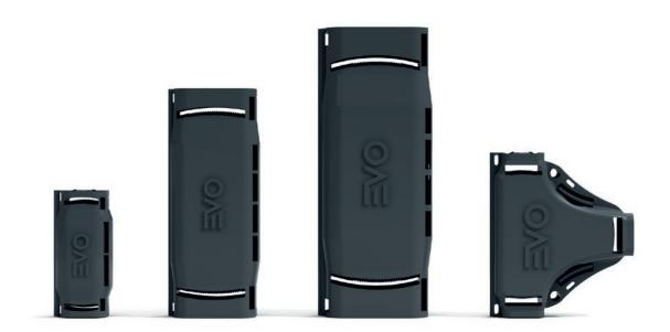
**EVO**<sup>®</sup> is the new range of gel-insulated joints, which allows straight and branch connections with **IP68 degree of protection** on the most widespread cable types in electrical wiring, with cross-sections up to up to  $5 \times 16 \text{ mm}^2$  (straight) and up to  $3 \times 4 \text{ mm}^2$  (branch).
