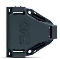
**EVO**<sup>®</sup> is the new range of gel-insulated connecting devices, which allows making straight and branch connections with **IP68 Degree of protection** on the widespread cable types in electrical wiring, with cross-sections up to  $3 \times 2.5$  mm<sup>2</sup>.
